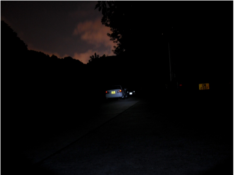
Penlight 0.5W LED 20 Lumen Note the 'bluish' shift of the white car.
