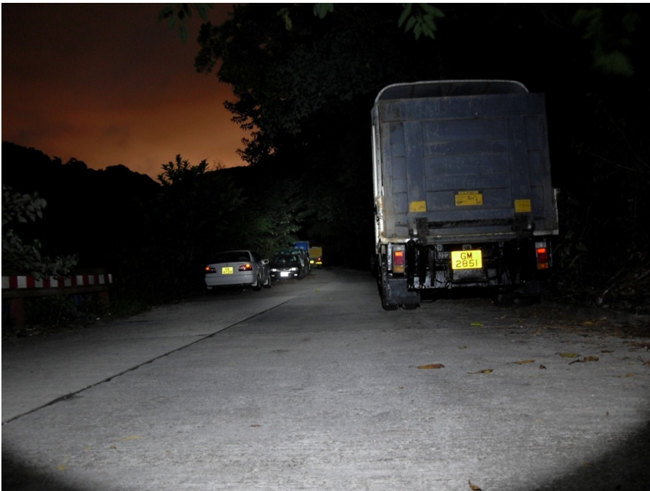
3W LED – 250 Lumen Shutter 8 & F2.8 (Notes: - Pila 'Quick-Switch' LED Emitter at 100% light output - Camera CCD responds to white LED better than to Xenon!)
